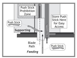
**Figure 69.** Using push sticks to rip narrow stock.
